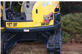
Yanmar pioneered the first zero tail swing excavator in 1993. Today, our true zero tail swing technology means no part of the housing extends beyond the tracks. Since the entire machine operates within its tracks, you can work efficiently almost anywhere with less damage to the machine and the worksite.
