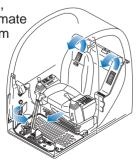
Cooling capacity: 4,8 kW (4,100 kcal/h) Heating capacity: 5,7 kW (4,900 kcal/h)
