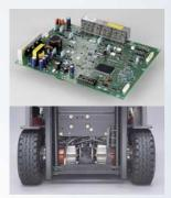
\* Power management of the twin drive motors and the pump motor for load handling and power steering is performed by full AC control. This AC Power System requires less maintenance cost than the current DC system.
