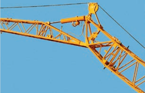
Adjustable folding jib (0° to 45°)
