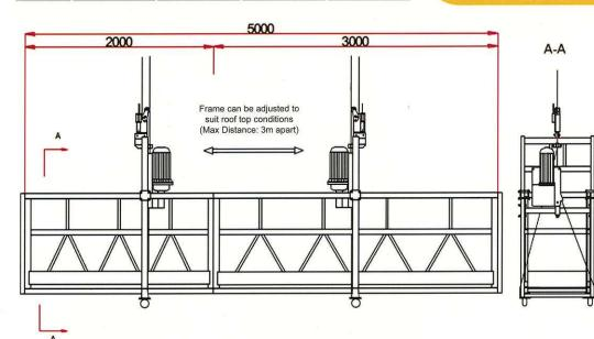
The modular gondola platform comes in standard lengths of 1m, 2m, 3m and can be assembled in various combinations to form a single length platform subject to an engineer's approval.
