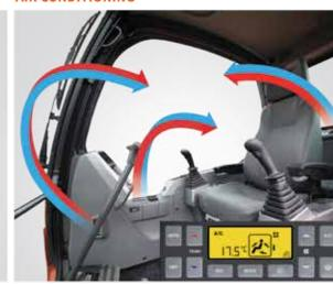
The high performance air conditioning provides an air flow which is adjusted and electronically controlled for the prevailing conditions. Five operating modes ensure even the most demanding operator will be satisfied.
