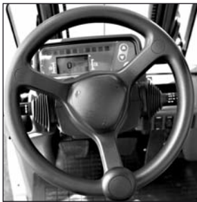
Fully hydrostatic steering
