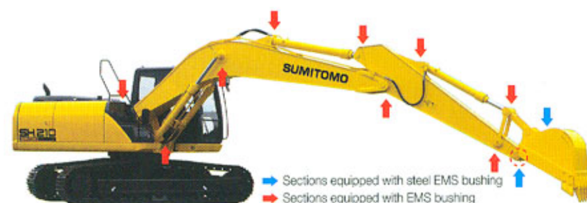
Steel EMS is installed around the bucket
