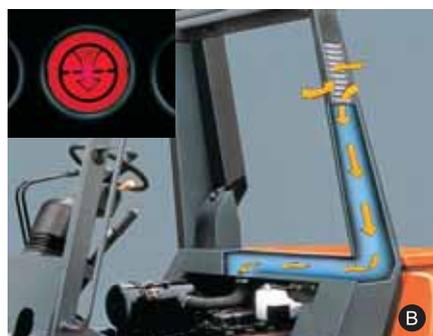
**B Air Intake:** To ensure a supply of clean air for the engine, a snorkel air intake is located on the upper porting of one of the pillars for the operator's headguard. An 8" cyclone air cleaner featuring outstanding air cleaning efficiency is used. A warning
