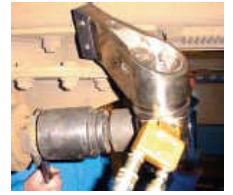
Patented Multi-Axis Swivel provides better accessibility and prevents hose kinking.
