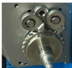
Double circlip winch with self-locking function
