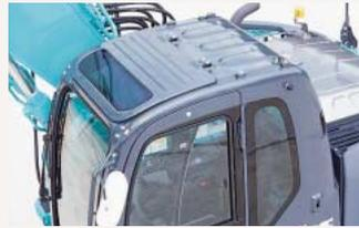
The ACERA GEOSPEC SR series has a safety rating equivalent to FOPS level 1. In addition to the standard roof guard, optional front and head guards are available. They can be easily attached with bolts to the standard cab brackets.
