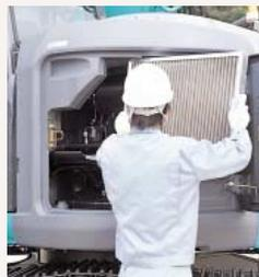
When checking and cleaning the cooling system, one must deal with several different components like the radiator, oil cooler and intercooler, which all must be handled in different ways. But with the iNDr filter, there's just one filter in one place. If it looks dirty during start-up inspection, it can be cleaned easily and quickly.
