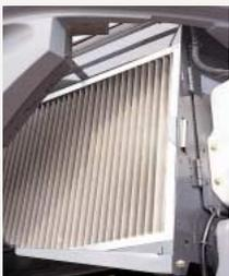
Outside air goes directly from the intake duct through the iNDr filter for dust removal. The filter features a 60-mesh screen, which means it has sixty holes per inch both vertically and horizontally, with a wide front surface area and accordion structure that resists clogging.
