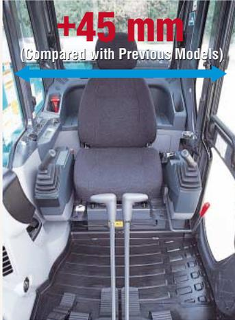
The new 'Big Cab' has the same width and height as the cabs installed on much larger machines. With more space to the front of the operator, it feels more roomy, and the larger area of floor space means greater comfort from the feet up. The operator has plenty of space in front for easy, comfortable operation, with ample foot room.
