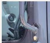
Easily repaired bolted handrails
