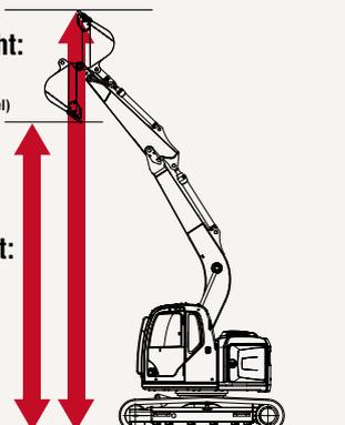
The bottom of the upper frame features single-plate construction for solid stability, combined with dramatic increases in maximum digging and dumping heights to deliver a wider working range than ever before.
