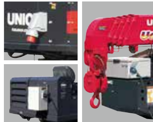
23 Electric power unit (AC200V or AC400V)
