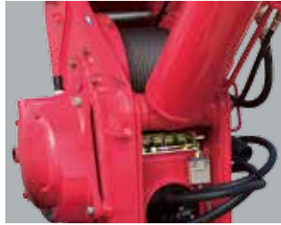
13 Automatic stop for leaving minimum wire rope
