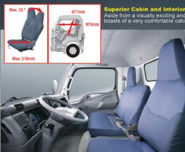
• Vinyl Seat Materials • 2-Spoke Urethane Steering Wheel • 3P ELR x2 and 2P Lapbelt x1 Seatbelts
